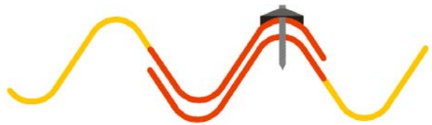
Figure 4. How to interlock tiles (1.5 to 2 curves) and how to fix tiles onto the crest to protect from water.
