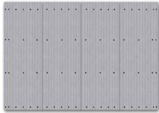
Figure 5. How to fix nails to binding tiles or corrugated sheets. For tile-tile connection, nails are fixed every 40 cm and for tile-structure connection, every 2 curves. For tiles on both ends of the roof, 2 nails are fixed on the first curves.
